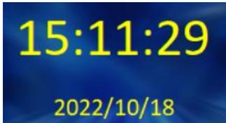
A yellow clock indicates that the PC has linked with the NTP-100S but the GPS is not working properly.
