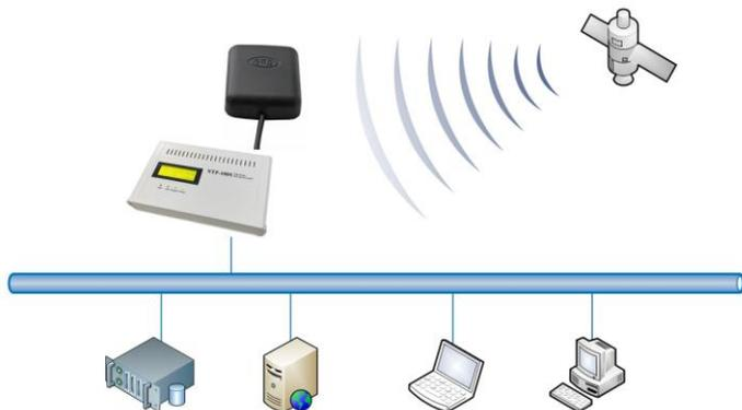
The NTP-100S Time Server is designed to provide very accurate time obtained from GPS satellites, so that all PCs in the same network can be precisely synchronized without accessing any outside NTP servers.
