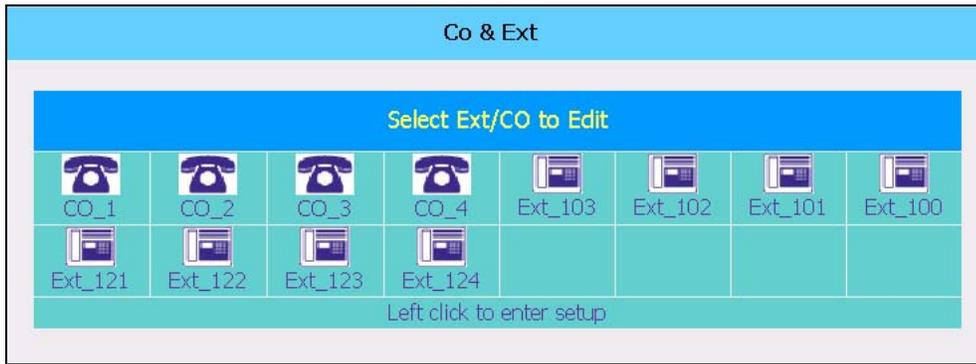
This menu lists all CO lines and extensions. However, it does not mean that all these lines have physical connections. For an unconnected or unused CO line, you should enter its setup menu and set its operation mode to “Disabled”. This way the system knows which CO line(s) should never be accessed.
